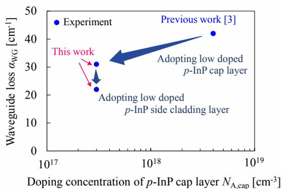
Fig. 5. The waveguide loss dependence on the doping concentration of  $p\text{-InP}$  cap layer.
