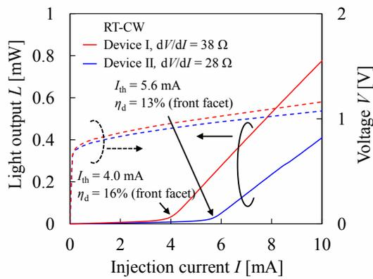
Fig. 3. Current–light output and current–voltage characteristics of membrane FP lasers. In case of the Device. I, a stripe width  $W_s$  and cavity length  $L$  are  $0.6 \mu\text{m}$  and  $830 \mu\text{m}$ , respectively. In case of Device. II,  $W_s$  and  $L$  are  $0.7 \mu\text{m}$  and  $900 \mu\text{m}$ .
