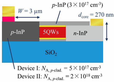
Fig. 1. Cross section of a membrane laser.
