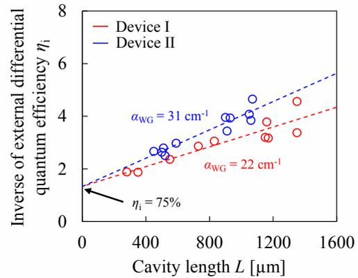
Fig. 4. Measured cavity length dependence of the inverse of the differential quantum efficiency.
