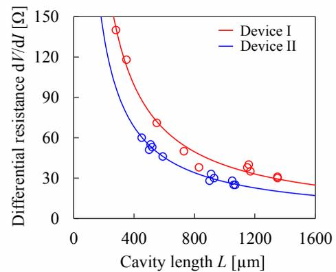
Fig. 6. Measured and fitting curve of cavity length dependence of the differential resistance.
