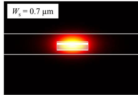
Fig. 2. Mode field profile of a membrane laser with a stripe width of  $0.7 \mu\text{m}$ .
