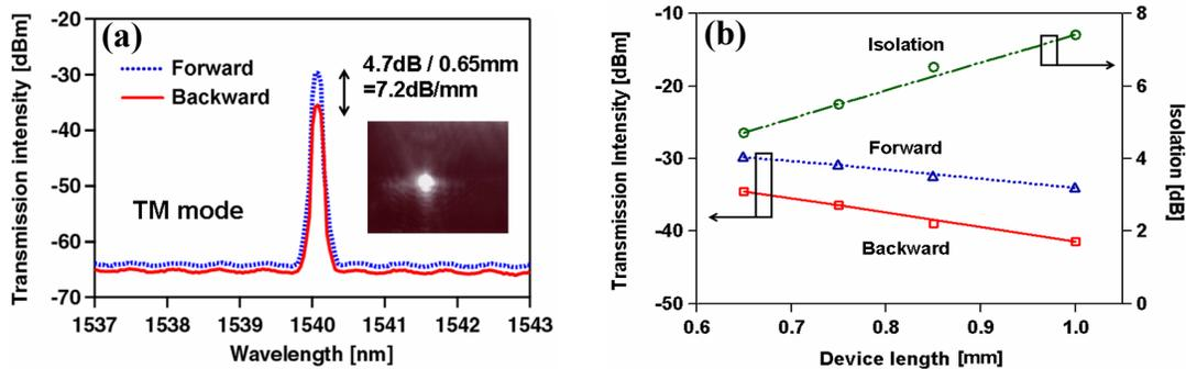
**Fig. 2** (a) Forward and backward transmission through the device with 0.65-mm length, measured for 1.54  $\mu\text{m}$  TM-mode light, with 100 mA driving current and 0.1 T magnetic field. (b) Transmission intensity and isolation ratio as a function of device length.
