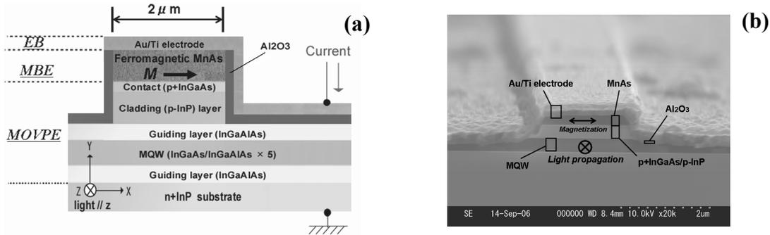
**Fig. 1** (a) Schematic cross section of the TM-mode waveguide optical isolator. The MnAs layer is magnetized along x-direction. Light passes perpendicular to the figure (z-direction). (b) Cross section of the device observed with a SEM.
