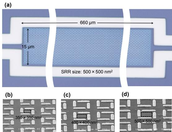
Fig. 3. (a) Optical microscope image of  $1 \times 1$  MMI with metamaterial consisting of  $500 \times 500 \text{ nm}^2$  gold SRR array. (b-d) SEM images of 4-cut SRR arrays with different sizes.
