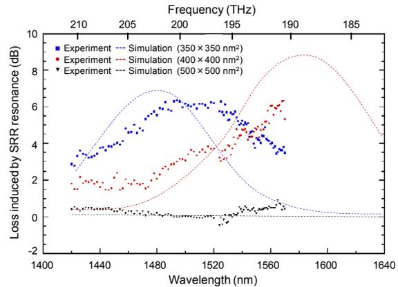
Fig. 4. Experimental propagation loss in devices with  $350 \times 350 \text{ nm}^2$  SRRs (blue dots), with  $400 \times 400 \text{ nm}^2$  SRRs (red dots), and with  $500 \times 500 \text{ nm}^2$  SRRs (black dots) as a function of wavelength from 1420 to 1570 nm, measured for TE-mode light. Simulation result is also plotted for each device (dashed lines).
