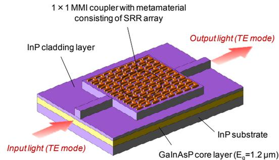
Fig. 1. Waveguide-based multimode-interferometer (GaInAsP/InP  $1 \times 1$  MMI) and metamaterial region (gold SRR array) attached on the waveguide.
