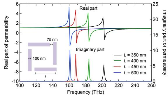
Fig. 2. Real and imaginary parts of permeability of gold SRRs in glass ( $\epsilon_r=2.25$ ) as a function of frequency, with SRR size  $L$  as a parameter ( $W_1 = W_2 = 100$  nm).
