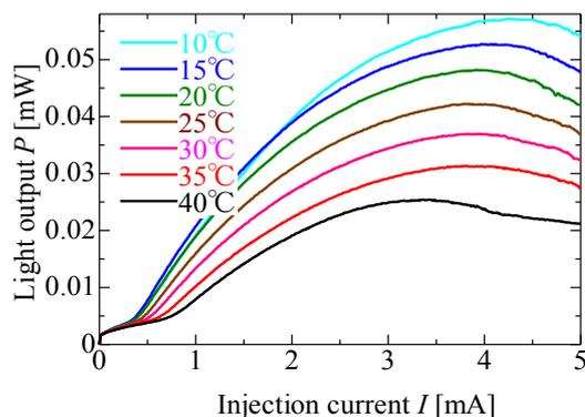
Fig. 4  $L-I$  characteristics at various temperatures ranging from 10 to 40°C.
