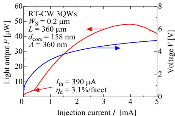
Fig. 3 Light output and  $V-I$  characteristics.
