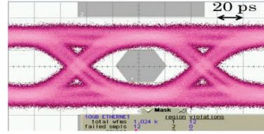
Fig.5 Eye diagram at 10 Gb/s( $V_{\text{bias}} = -2 \text{ V}$ ).
