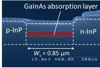
Fig. 3 Cross sectional SEM view of the lateral junction structure.
