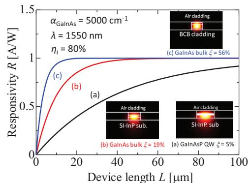
Fig.2 Responsivity dependence on the device length
