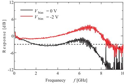
Fig. 4 Frequency response with various bias voltage.
