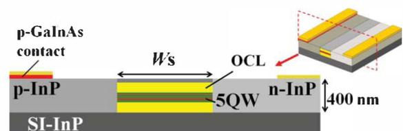
Fig. 1 Cross-sectional structure of LCI lasers on SI-InP.
