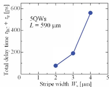
Fig.4 Stripe width dependences of carrier injection delay.
