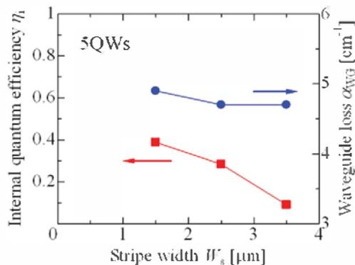
Fig.3 Stripe width dependences of internal quantum efficiency and waveguide loss.
