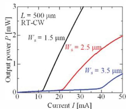
Fig.2 Lasing characteristics of LCI laser for various stripe widths.
