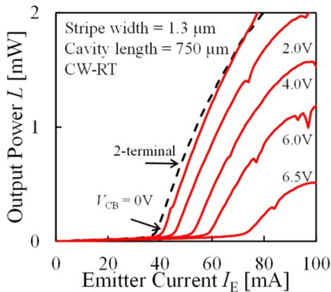
Fig. 3 Lasing characteristics of the TL under common base configuration.
