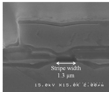
Fig. 2 SEM view of fabricated device.
