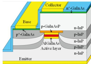
Fig. 1 The structure of fabricated npn-AlGaInAs/InP TL.
