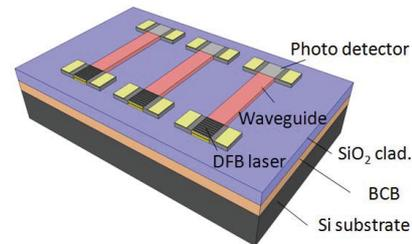
Fig. 1 Schematic representation of membrane photonic integrated circuits.
