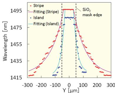
Fig. 4 Peak wavelength distribution depending on the distance from the mask center.
