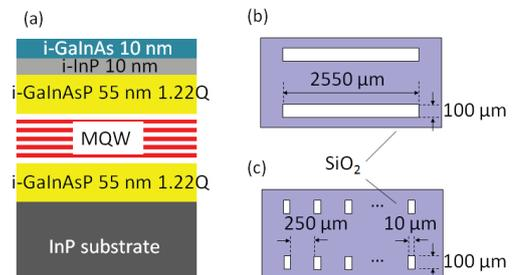
Fig. 2 (a) Epitaxial base structure with 5 quantum-well active region of 90 nm, (b) QWI-SiO<sub>2</sub> masks margin stripe type, and (c) island type.
