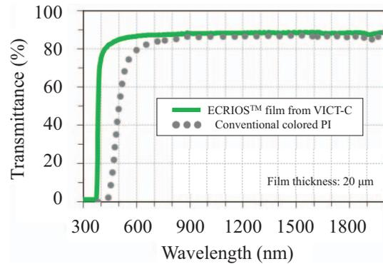
Fig. 2. Measured transmission spectra of ECRIO<sup>TM</sup> film.
