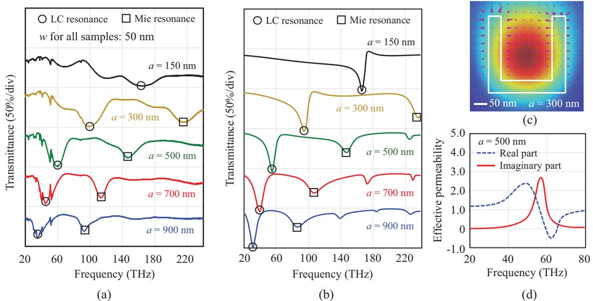
Fig. 3. Measured (a) and calculated (b) transmission characteristics of metafilm with different ring size. (c) Magnetic field distribution around ring (arrow: electric field). (d) Retrieved effective relative permeability of metafilm with 500-nm ring.
