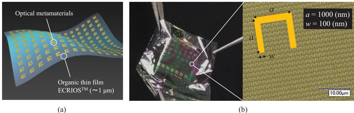
Fig. 1. (a) Schematic image of metafilm. (b) Optical microscope image of metamaterial array embedded in organic thin film.
