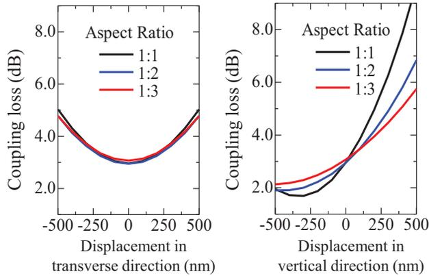
Fig. 2 Calculation result of the mode coupling loss between PWB and LCI laser regarding different aspect ratio with tolerance characteristic in both direction.
