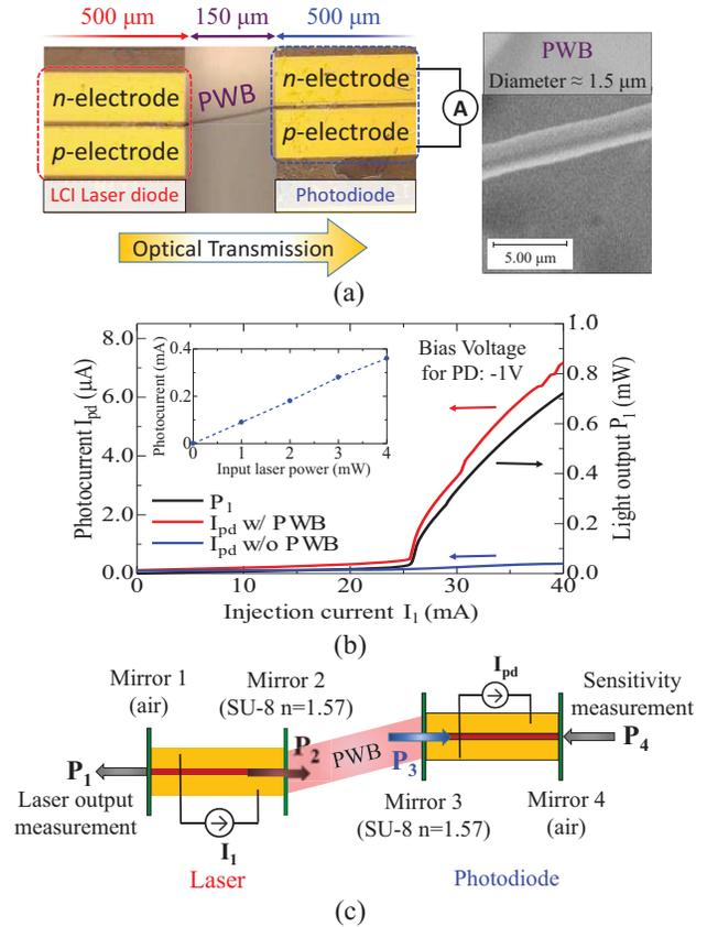
Fig. 3 (a) Optical microscope image of the completed sample. (b) Measured photocurrent  $I_{pd}$  of the photodiode regarding of the injection current to laser  $I_1$  together with the laser I-L characteristic. The inset shows the property of an individual PD. (c) The schematic figure of optical transmission between laser and photodiode chips.
