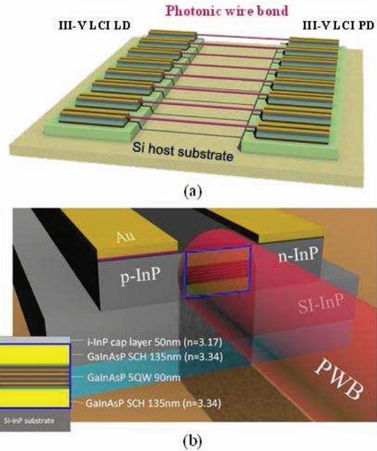
Fig. 1 (a) Concept of optical interconnection between two LCI optical chips based on photonic wire bonding. (b) Details of the transition section between the LCI laser and PWB.
