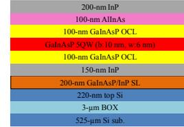
Fig. 1. wafer structures for oxidation processes.
