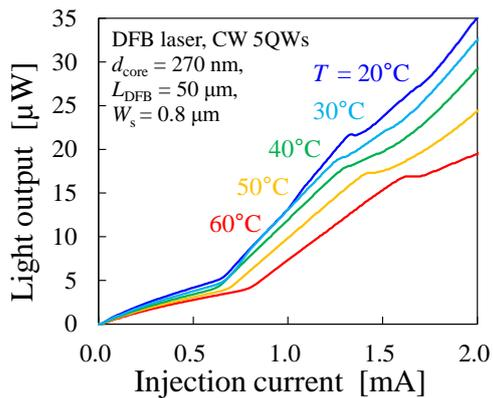
Fig. 5. Light output characteristics of membrane DFB laser for various temperatures.
