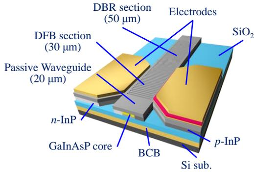
Fig. 1. Schematic structure of a membrane DR laser.
