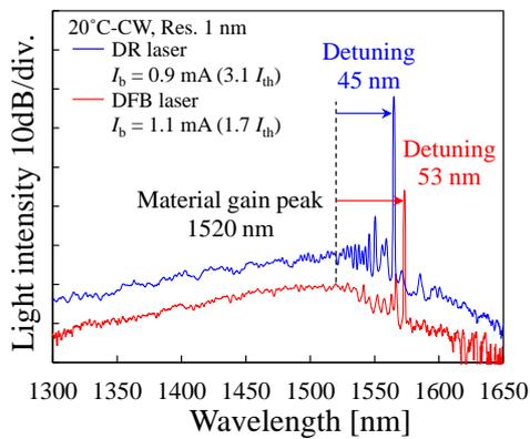
Fig. 3. Emission spectra of membrane DR and DFB lasers.
