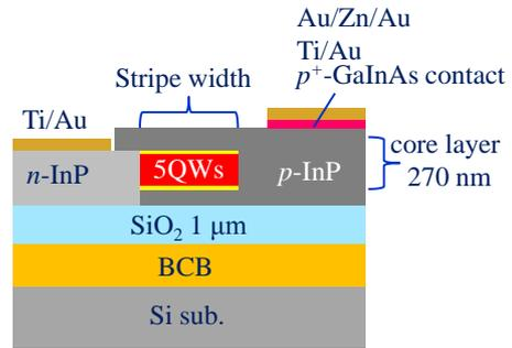
Fig. 2. Cross section at DFB section of fabricated devices.
