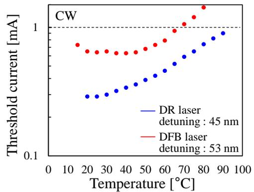
Fig. 6. Threshold current of membrane DR and DFB lasers as a function of temperature.
