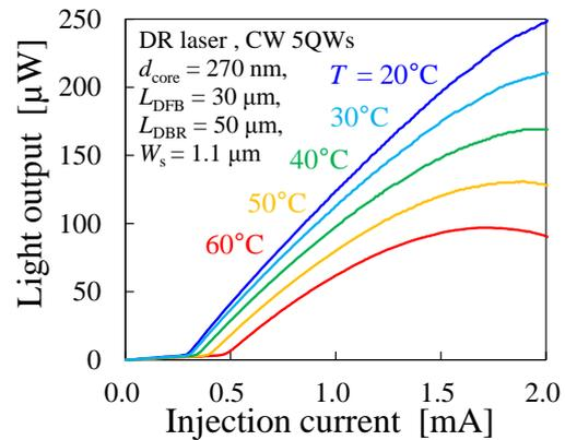
Fig. 4. Light output characteristics of membrane DR laser for various temperatures.
